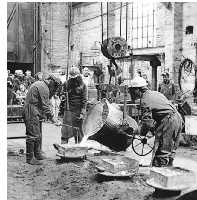
The casting of two new bells by Taylors of Loughborough. A new Treble and Second, March 4th 1999.
